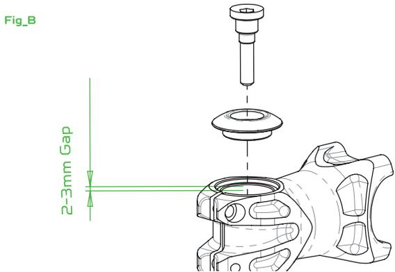
**003\_**Re install the two greased steerer tube clamp bolts and slightly tighten them. When you are happy with the stem orientation (making sure the stem is in line with the front wheel), tighten alternately the steerer tube clamp bolts to **5 N.m**
