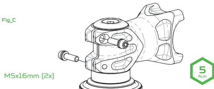
**004\_**Install the handlebars and position the clamp. First install the two top clamp bolts (previously greased) and slightly tighten them. When you are satisfied with the handlebars position, tighten the two top clamp bolts to **5 N.m**. Alternate between the two bolts when tightening until torque setting is achieved.
