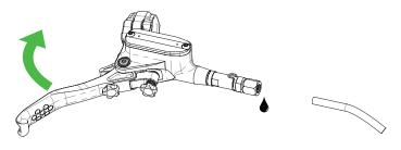
OO7\_Press the brake hose into the coupler - there should be a full 8mm of insertion. While holding the coupler with a 8mm spanner use a 10mm to carefully tighten the nut on the coupler until there is **NO GAP**. When tightening make sure to keep the coupler straight being careful not to bend the retaining clip.
