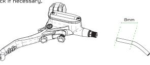
**004\_**Using a 8mm spanner, unscrew the straight connector and keep the M6 copper washer aside.
