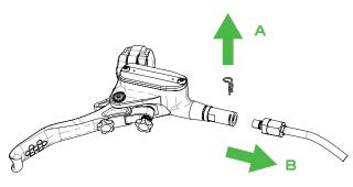
INSPECT THE RETAINING CLIP: If bent or damaged it MUST be replaced
