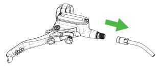
**002\_**Pull back the shroud and cut the hose clean just behind the olive. Be careful not to cut through brass insert. Then remove the shroud.
