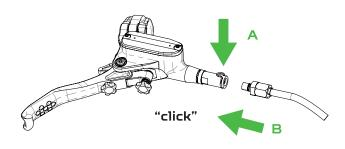
**003**\_Gently pull on each brake hose to check the connection is secure.
