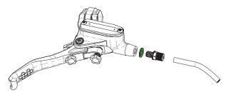
**005\_**Install the Quick Connector unit and M6 copper washer. thread initially by hand and tightening using a 8mm spanner.
