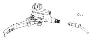
**003\_**You **must** have at least 8mm of clean, straight hose to further install the coupler. Make sure the internal diameter of the hose is clean and not pinched, open up with a straight pick if necessary.
