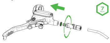
**005**\_Gently and slowly pull the brake lever until one single drop of brake fluid comes out of the speed connector assembly. You may need to pump several times.
