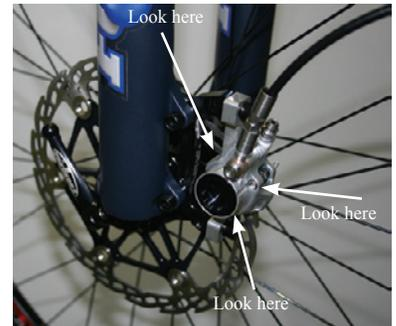
repeatedly. See which piston is working the most/least. It should be fairly obvious and you may see the rotor being 'pushed' over whilst operating the brake
