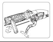
Finger reach adjustment : The Mini lever allows the adjustement of the lever reach. This refers to the position of the lever blade relative to the bars.
