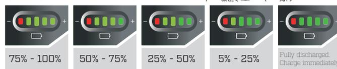
The ES (Energy Status) battery pack features a 5 stage fuel gauge. Press and hold the 'TEST' button to activate the LED display. This gives a visual indication of the remaining capacity within the battery cells.
