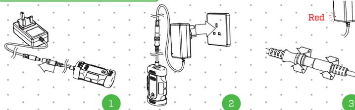
**DANGER:** Use only the 7.4v Li-Ion battery pack supplied with the lighting system. Any attempt to use or charge another battery pack may result in explosion and serious injury.
