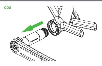
**002\_**Keep turning the bolt in an anticlockwise direction, it will go loose and then you will feel resistance as the crank starts to extract off the axle, keep turning until the drive side crank comes right off the axle.
