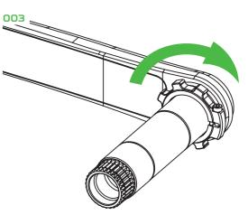
**003\_**Slide the non drive side crank assembly out of the bottom bracket.
