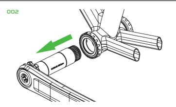
**002\_**Keep turning the bolt in an anticlockwise direction, it will go loose and then you will feel resistance as the crank starts to extract off the axle, keep turning until the drive side crank comes right off the axle.
