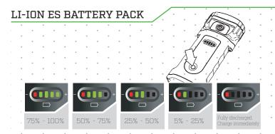
The integrated ES (Energy Status) battery features a 5 stage fuel gauge. Press and hold the 'TEST' button to activate the LED display. This gives a visual indication of the remaining capacity within the battery cells.
