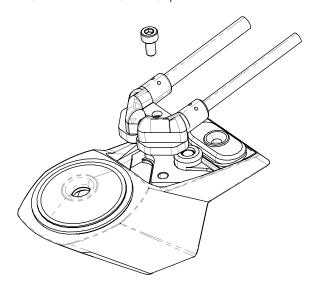
**004\_**Using a 2.5mm Allen key, remove M4 countersunk screw to release the display connection plate.
