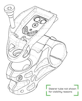
**007\_**Re-install the KIOX display computer. If you are using the securing screw it may need to be installed prior to fastening the mount onto the stem.
