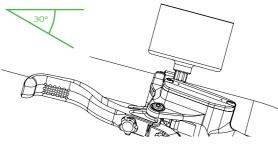
012\_Rotate the bike in the stand so the lever end of the master cylinder points upwards around 30° and repeat step O11.
