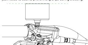
005\_Rotate the master cylinder (M/C) so that the top of the bleed funnel sits in a level position. This position orientates the brake so that air will naturally rise out of the sustem during bleeding.
