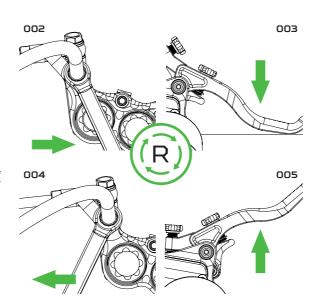
NOTE: Do not release the brake lever with the caliper bleed nipple open, this will draw air back into the system.
