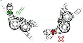
003\_Make sure the caliper bleed nipple is positioned on the top of the caliper. Usually front calipers can remain attached to the bike while rear calipers should be removed and dropped below the bike. This is especially important where rear hose routings create a dip around the bottom bracket area; try to position the caliper so it sits at the lowest part of the sustem to avoid creating an air trap.
