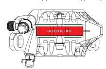
002\_Push the caliper pistons all the way back into the housing.
