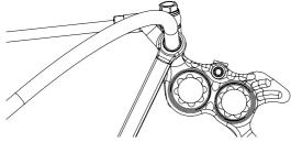
008\_Fit an 8mm spanner over the caliper bleed nipple and then push on either the bleed kit nipple adapter/hose or any piece of appropriate diameter clear hose. Route the other end of the hose into a waste bottle or jar.
