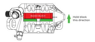
006 With the bleed nipple closed, pump the brake lever to move the pistons out of the caliper. Hold the piston/ pistons on one side of the caliper back in the housing, using a flat blade screwdriver against the bleed block or pads, so that the opposite pistons come all the way out to contact the bleed block.
