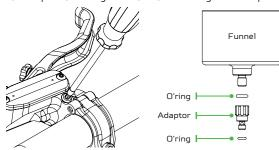
004\_Remove the master cylinder bleed port screw using a T10 Torx driver. By hand, screw the EVO bleed port adapter onto the bleed funnel, don't be tempted to over tighten the adapter or use any tool. Thread the funnel/adapter assembly directly into
