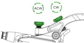
007\_Position the lever adjustments so both reach and bite point are fully out (reach adjuster turned fully clockwise and bite point adjuster turned fully anti-clockwise)
