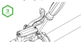
005\_Clean up any residual brake fluid left on the brake using warm soapy water.
