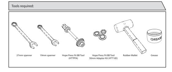
We strongly advise that this bottom bracket is installed and maintained by a competent cycle mechanic, using Hope Press Fit BB Tool (HTTPFA) with the 30mm Adapter Kit (HTT185).
