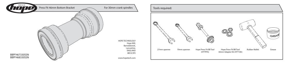
We strongly advise that this bottom bracket is installed and maintained by a competent cycle mechanic, using Hope Press Fit BB Tool (HTTPFA) with the 30mm Adapter Kit (HTT185). This bottom bracket is intended for installation in bottom bracket shells with an internal diameter of 46mm and widths of 73mm or 83mm.
