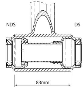
1. Install the drive side cup (with bearing fitted).
