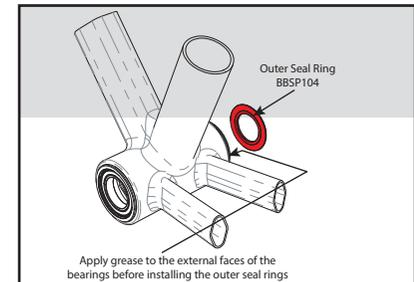
Your bottom bracket is now fully installed and ready for the continued installation of your crank set.
