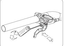
Use a 2mm Allen key, turn the adjuster screw clockwise to increase the reach and anticlockwise to reduce it.
