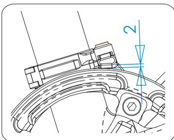
3. Make sure the seat tube is clean and free of any dirt or mud. Install the clamp around the seat tube and slightly tighten the M4 cap screw but still allow the clamp to slide up and down.
