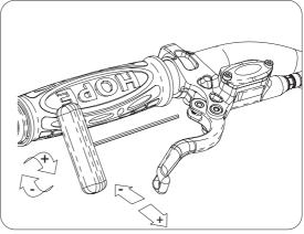
Finger reach adjustment: The Mini lever allows the adjustement of the lever reach. This refers to the position of the lever blade relative to the bars. Use a 2mm Allen key, turn the adjuster screw clockwise to increase the reach and anti-clockwise to reduce it.
