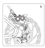
On IS mounts you will have to use an adaptor bracket to be able to fit the brake caliper.
