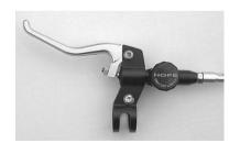
Under no circumstances should you use a Closed system caliper with an Open system lever (and vice versa). A mismatched system will not work and result in brake failure.
