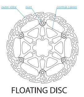
To avoid any permanent deformation even under the most severe conditions, a floating disc is constructed in two parts. An aluminium centre part (carrier) which is fixed to the hub and a stainless rotor part in contact with the brake pads. This is a high performance type brake disc.
