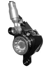
The Mono M4 caliper - A caliper with 4 pistons. The
